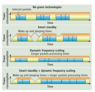
Improving efficiency. Packet service times and power consumption when no green technologies are applied, with only smart standby, with only dynamic frequency scaling, and with both smart standby and dynamic frequency scaling.
