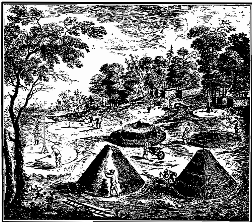
BEFORE THE ADVENT OF COAL wood was the main source of heat energy in Europe. Industrial power was provided by wind, animals and running water. It was often necessary to convert the wood to charcoal by partially burning it in furnaces such as the ones shown here. The wood was piled in stacks, covered with earth and powdered charcoal dust and then burned. The covering kept combustion at a minimum so that the end product was charcoal rather than ashes. For some manufacturing processes charcoal was preferred to wood because it is mostly pure carbon and so yields a greater amount of heat per unit volume of fuel. Illustration is from Diderot's Encyclopédie, ou Dictionnaire Raisonné des Sciences, des Art et des Métiers .
